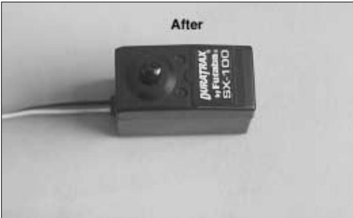
❑ 2. Using a pair of sharp cutters or a hobby knife remove the servo mounting tabs on both ends of the servo as shown above. Make sure the area where the mounting tabs were located is flush with the case when you are done. This will provide a good contact surface for the servo to mount.
