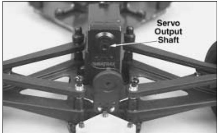
❑ 4. Install the servo onto the chassis, securing it in place with the double-sided tape. **Note: The servo needs to be mounted so that the output shaft is in the upper position as shown.**
